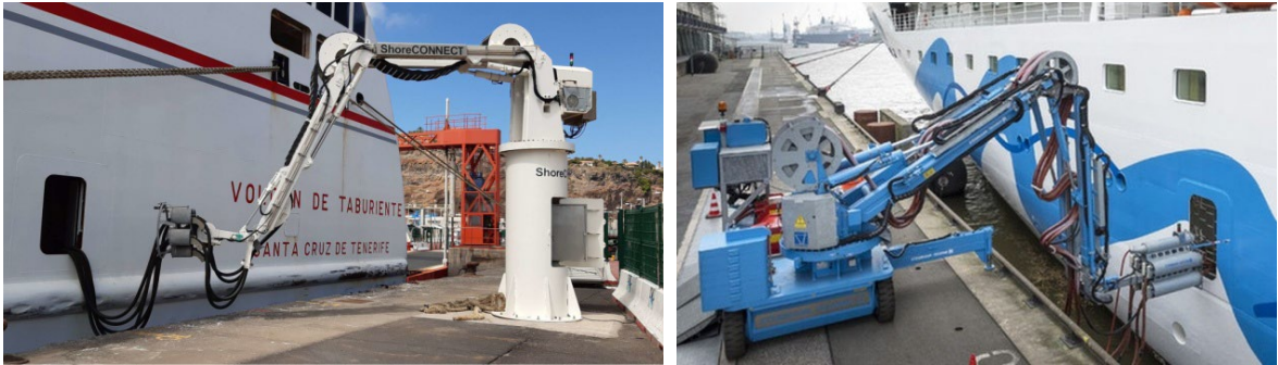
Fig.3 Shore power supply systems
